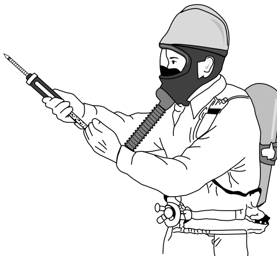
Applicator wearing an air pack (SCBA) and using a piston-type gas detection device.
