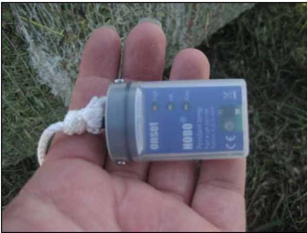
Figure 2. Temperature data loggers
