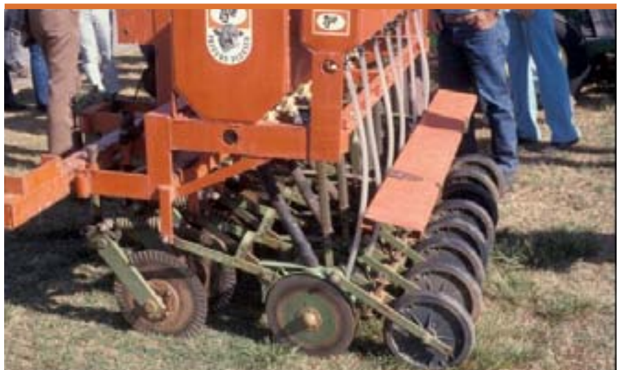
Figure 12-33. A grassland drill can be used for seeding legumes and grasses into grass sods or small grain stubble. Note that it has a coulter for slicing the soil, openers to make a place to deposit the seed and press wheels for getting soil-seed contact.
