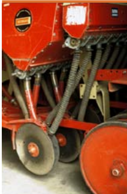
Figure 12-32. For successful seeding of small-seeded legumes and grasses with a grain drill, risks are reduced if the drill has a small-seeded legume box, tubes which deliver the seed behind the coulters and press wheels that increase soil-seed contact.
