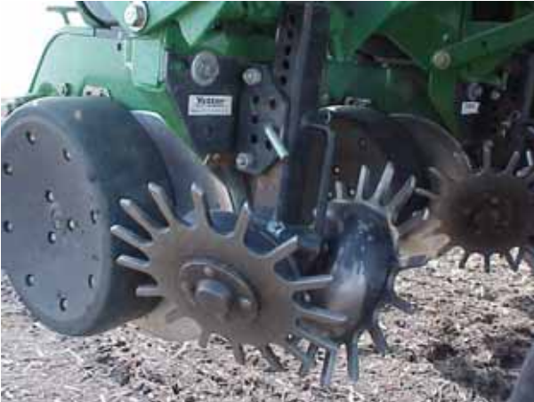
Photo 7. Residue managers on the planter to clear the row.
