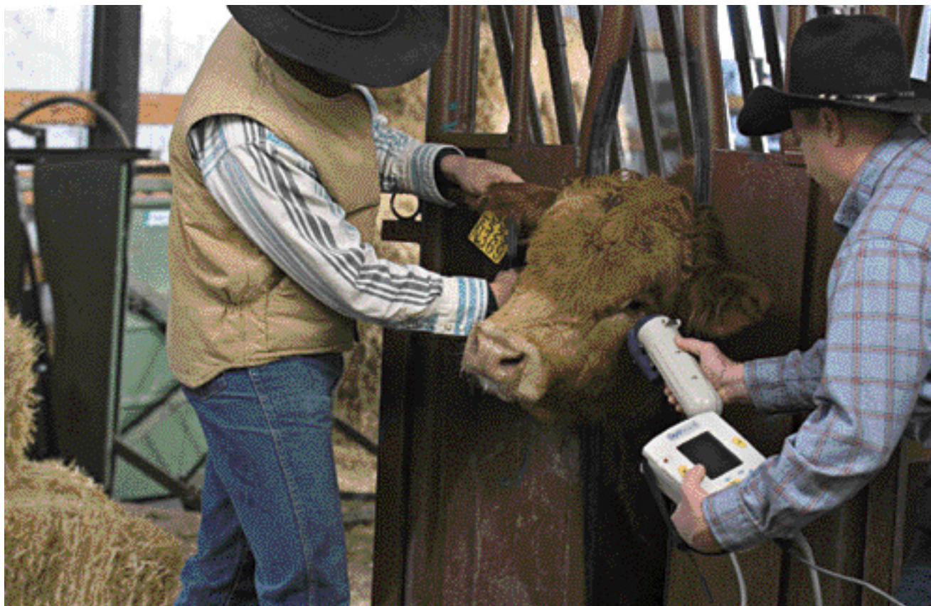
The OptiReader scans an animal's eye to capture an image of the retinal vascular pattern.
