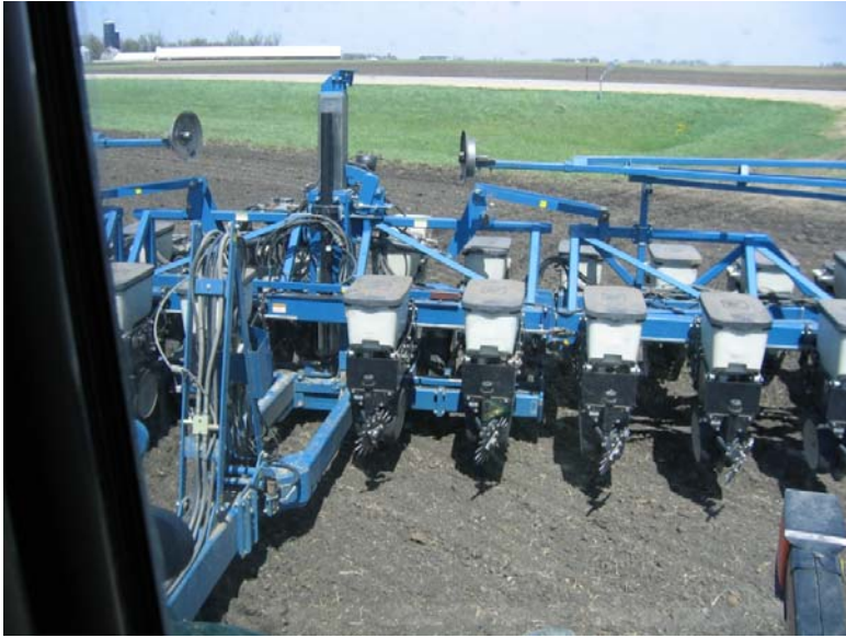
Figure 1: Twin-row planter used at the Wilmont, MN site in 2010.
