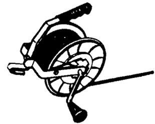
Reels with steel cranks cost about \$10 more than reels with plastic cranks. Spend the money. A reel should be able to take a little abuse, after all this is for use on a farm, not a china shop.
